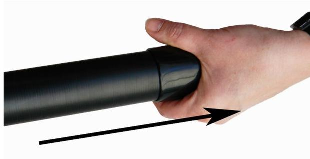
Open the lever on the extension and slide it on from the base of the pole. Fully slide the section up the pole and close the clamp lever. You will need to slide the pole hose up from the base of the pole and re-connect to the gooseneck fitting before re-attaching the gooseneck.
