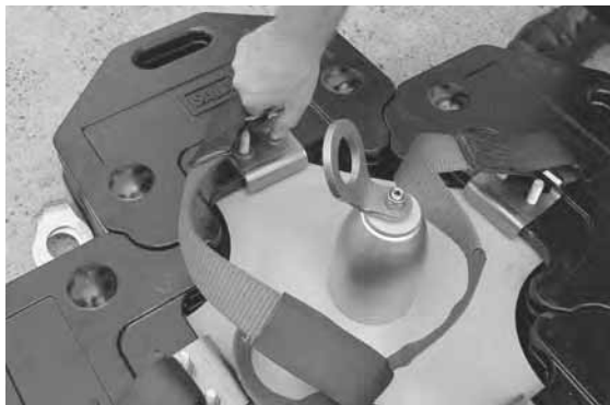
Figure 13 - Place Lifting Kit Brackets on U-Bolts
